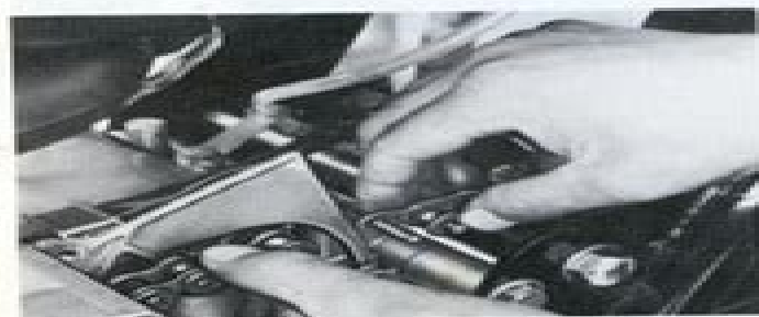
Fig. 8-1-7 Detaching chain joint
