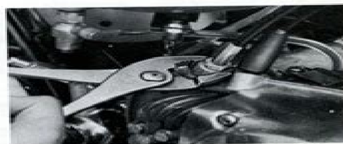
Fig. 8-1-10 Removing engine tachometer cable
