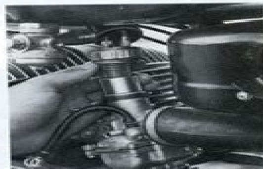
Fig. 8-1-8 Pulling throttle valve out of carburetor
