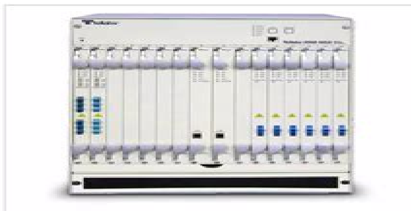
The Tellabs 5500 NGX-S switch combines integration of DCS, transport and data technology.
