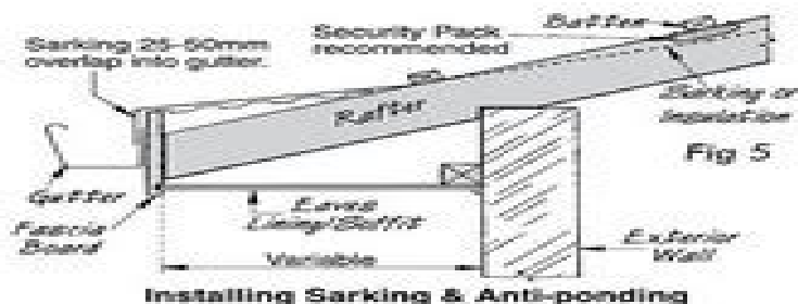
Installing Sarking & Anti-ponding
